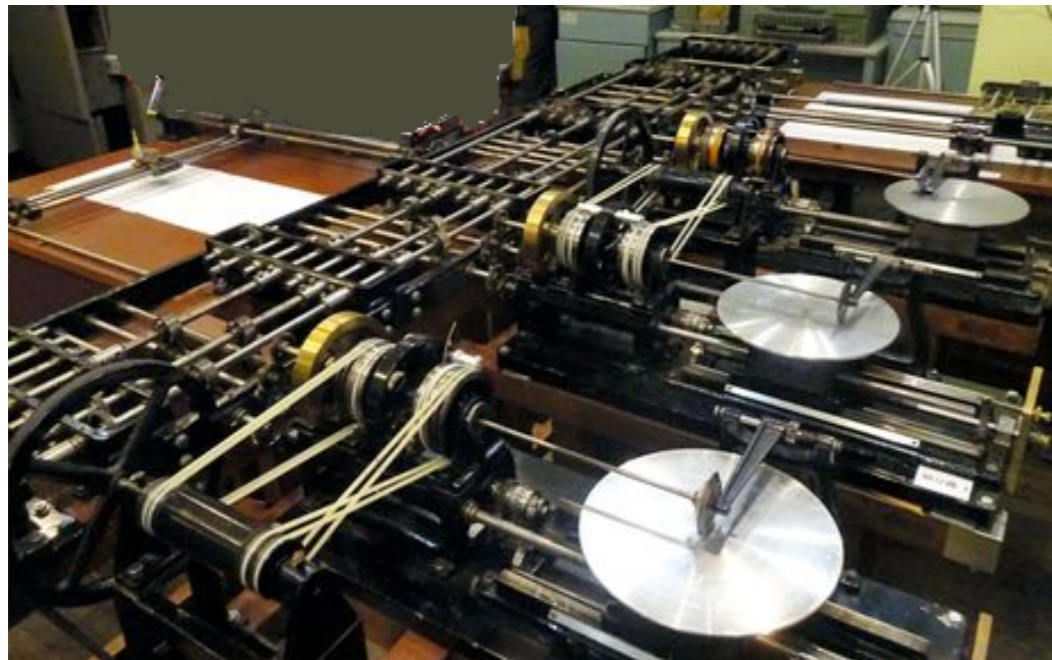
Differential analyzer 1920-40s
